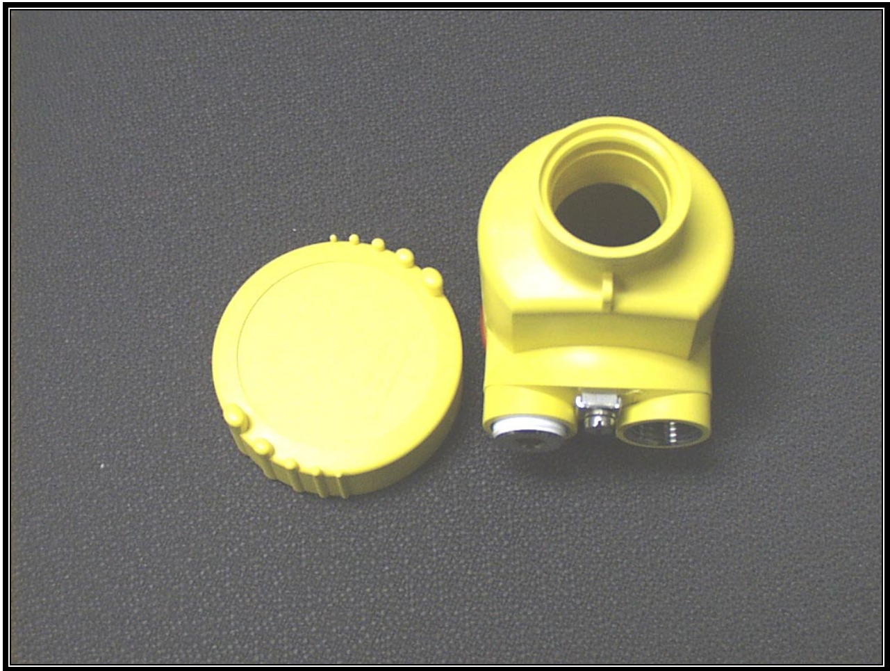
PHOTOGRAPH 6: EUT PLASTIC HOUSING FITTING
