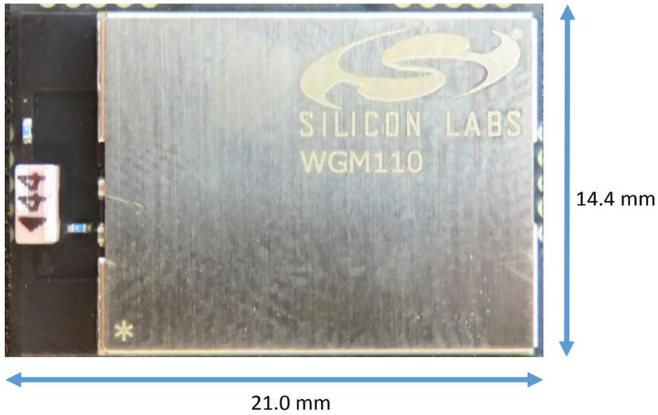
Figure 1: WGM110 External Photo, top view
