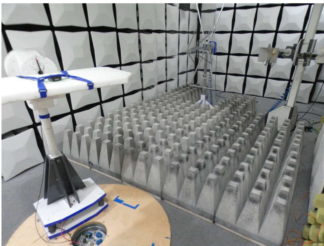
Photo 3: Setup Spurious Emissions Radiated (FAC), > 1GHz
