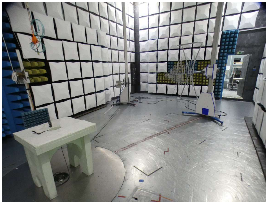
Photo 2: Setup Spurious Emissions Radiated (SAC), < 1 GHz, EUT vertical
