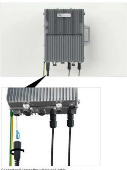
Connect and tighten the waterproof cable ( waterproof sleeve to be purchased separately) to MP-PS.
