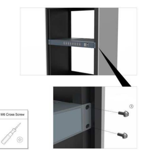
Install the AU-PS into the 19" rack and fasten with 4×M6 screws.
