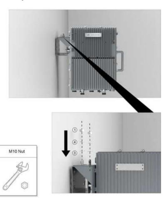
Hang the MP-PS on the mounting bracket | and fasten with 2=M10 nuts.
