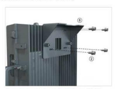
Faster the mounting bracket I to the back of MP-PS with 4×M16×14 screws.
