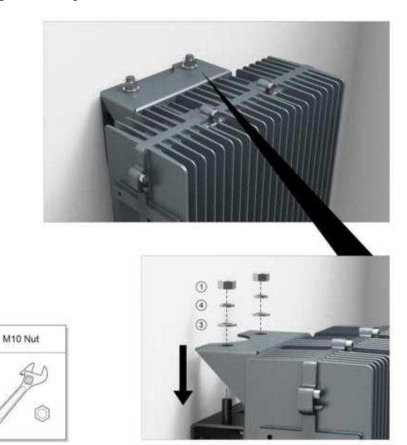
Hang the MP-PS on the mounting bracket  $\,I$  and fasten with  $\,2\!\times\!M10$  nuts.
