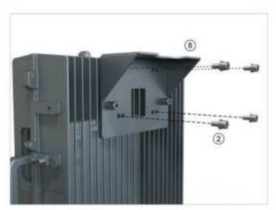
Fasten the mounting bracket I to the back of MP-PS with 4×M16×14 screws.
