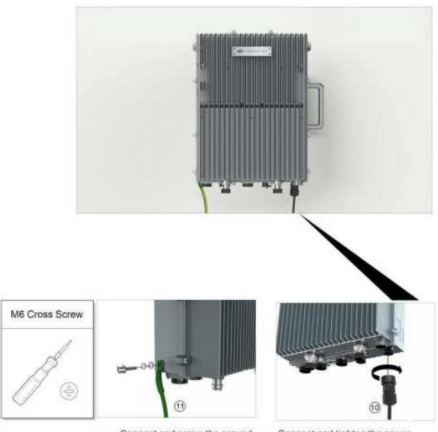
Connect and screw the ground wire to MP-PS.
