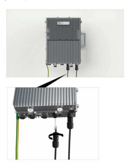
Connect and tighten the waterproof cable (\* waterproof sleeve to be purchased separately)to MP-PS.
