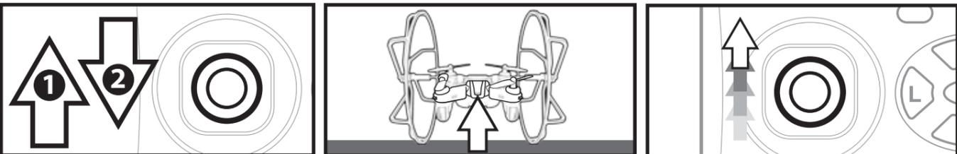
**EN** 4. Push the throttle level up to the maximum position (1) and back to minimum position (2) to complete the connection.
