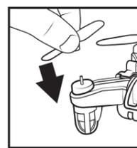
**CAUTION:** Rotor to be replaced by adult only. **NOTE:** If hair or debris gets caught in rotor and prevents rotor from turning, remove and clean.
