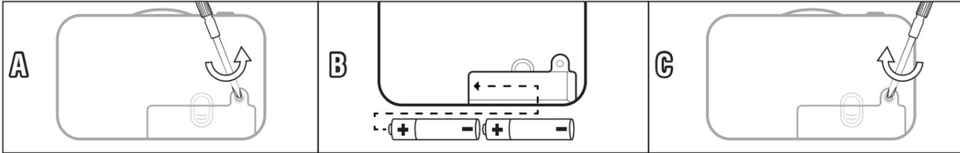
**EN** 1. Open the battery door with a screwdriver (A). 2. If used batteries are present, remove these batteries from the unit by pulling up on one end of each battery. DO NOT remove or install batteries using sharp or metal tools. 3. Install new batteries as shown in the polarity diagram (+/-) inside the battery compartment (B). 4. Replace battery door securely (C). 5. Check your local laws and regulations for correct recycling and/or battery disposal.
