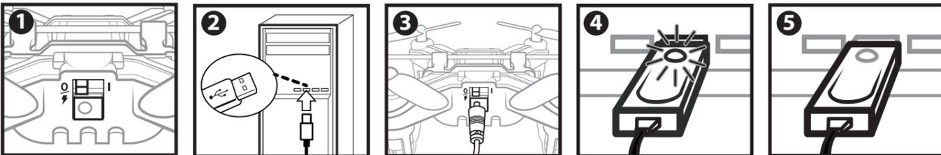
**EN** 1. Turn off the vehicle. 2. Plug the USB cable into a computer. 3. Carefully plug the other end of the USB cable into the vehicle. 4. The Charging Indicator will blink RED when charging. 5. The Charging Indicator will turn OFF when fully charged. 6. Once fully charged, remove the charging wire.
