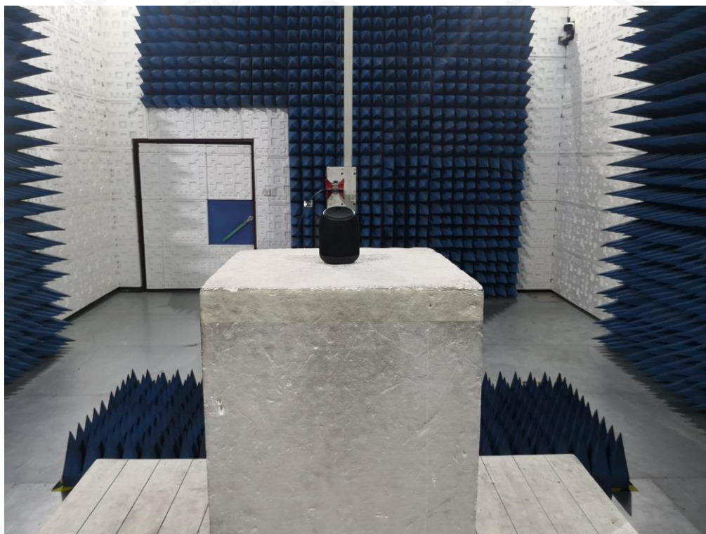
RADIATED EMISSION TEST SETUP ABOVE 1GHZ
