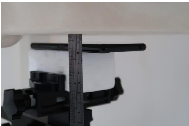
Front, Test Separation 10 mm
