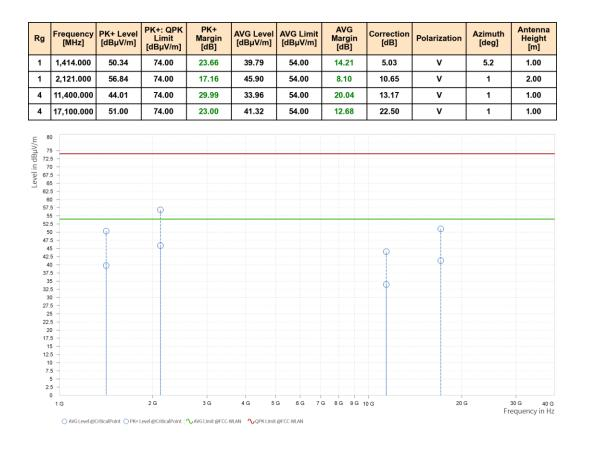
Note: For frequency above 18GHz, the emission was tested 20db below the limit so the data not recorded in the sheet.
