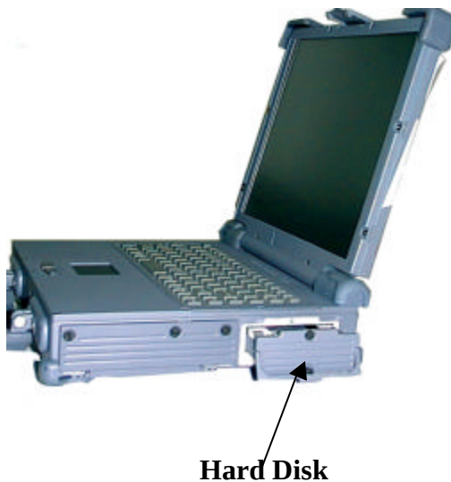
Figure 2-7 Removing a Hard Disk
