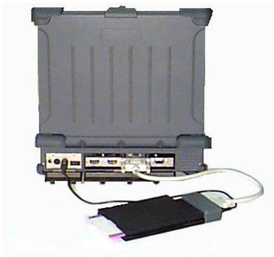
Figure 2-9 Use the External FDD
