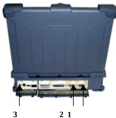
Figure 2-3 Connecting the External Power, Serial , and Parallel ports
