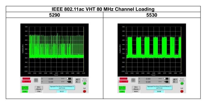
Note: During the monitoring period of 100ms, the packet flow exceeds 17%
