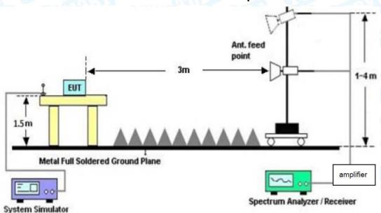
**Above 1GHz Test Setup**
