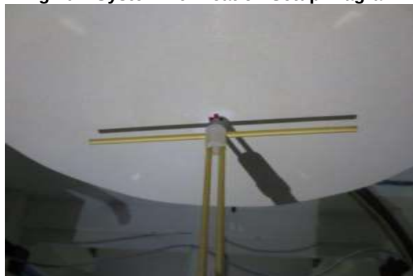
Fig.10.2 Photo of Dipole setup
