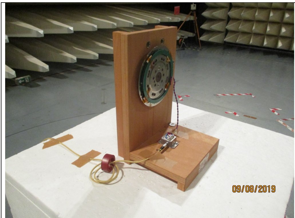
Photograph A2-3: EUT with stator unit connected with connection cable and ferrite with 3 turns
