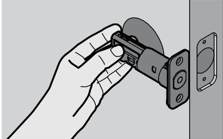
Hold the latch in front of the bore hole, with the latch face flush against the door edge. Is the slotted hole centered in the door hole?
