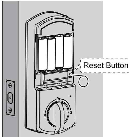
**C** If the reset is successful, the latch bolt will extend on its own to learn the handing orientation of the door.
