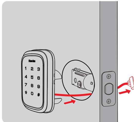
C Secure the mounting plate with the supplied screws. Do not overtighten screws.
