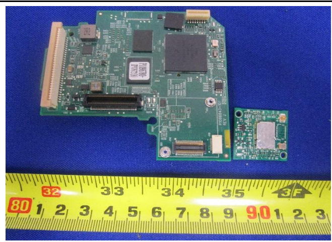
PCBA 2 Top View without radio module
