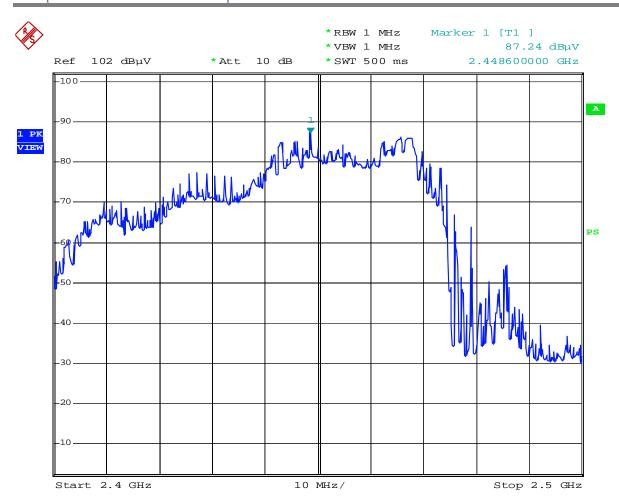
Whirlpool Microwave Oven GH4155 Frequency Stability VS Voltage End
