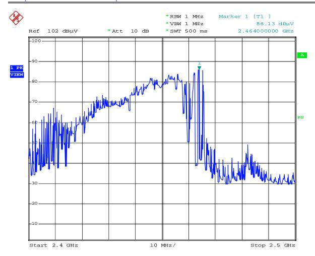
Whirlpool Microwave Oven GH4155 Frequency Stability VS Volta ge Start
