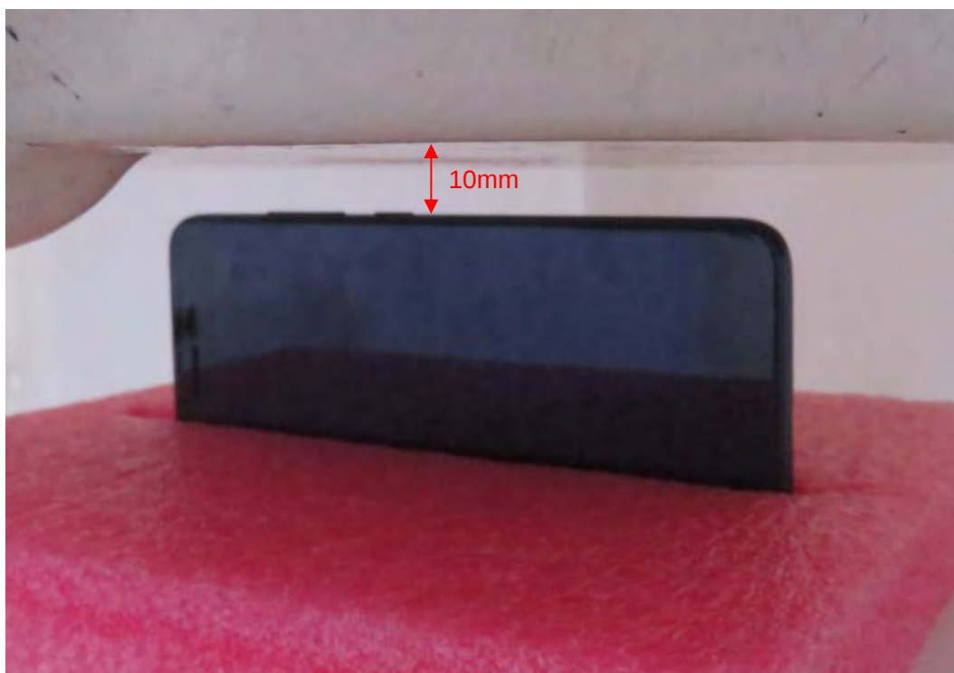
Picture 25: Right Side, the distance from handset to the bottom of the Phantom is 10mm
