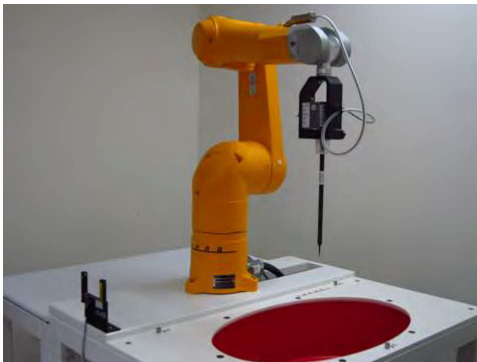
Fig.1 Photograph of the SAR measurement system
