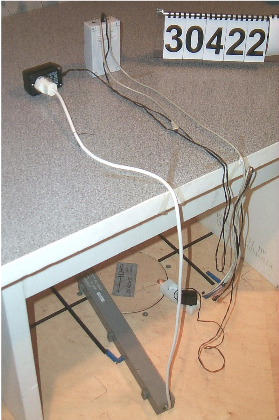
30422_a.jpg Model 24W test set-up preliminary emission measurement (9 kHz to 1 GHz)
