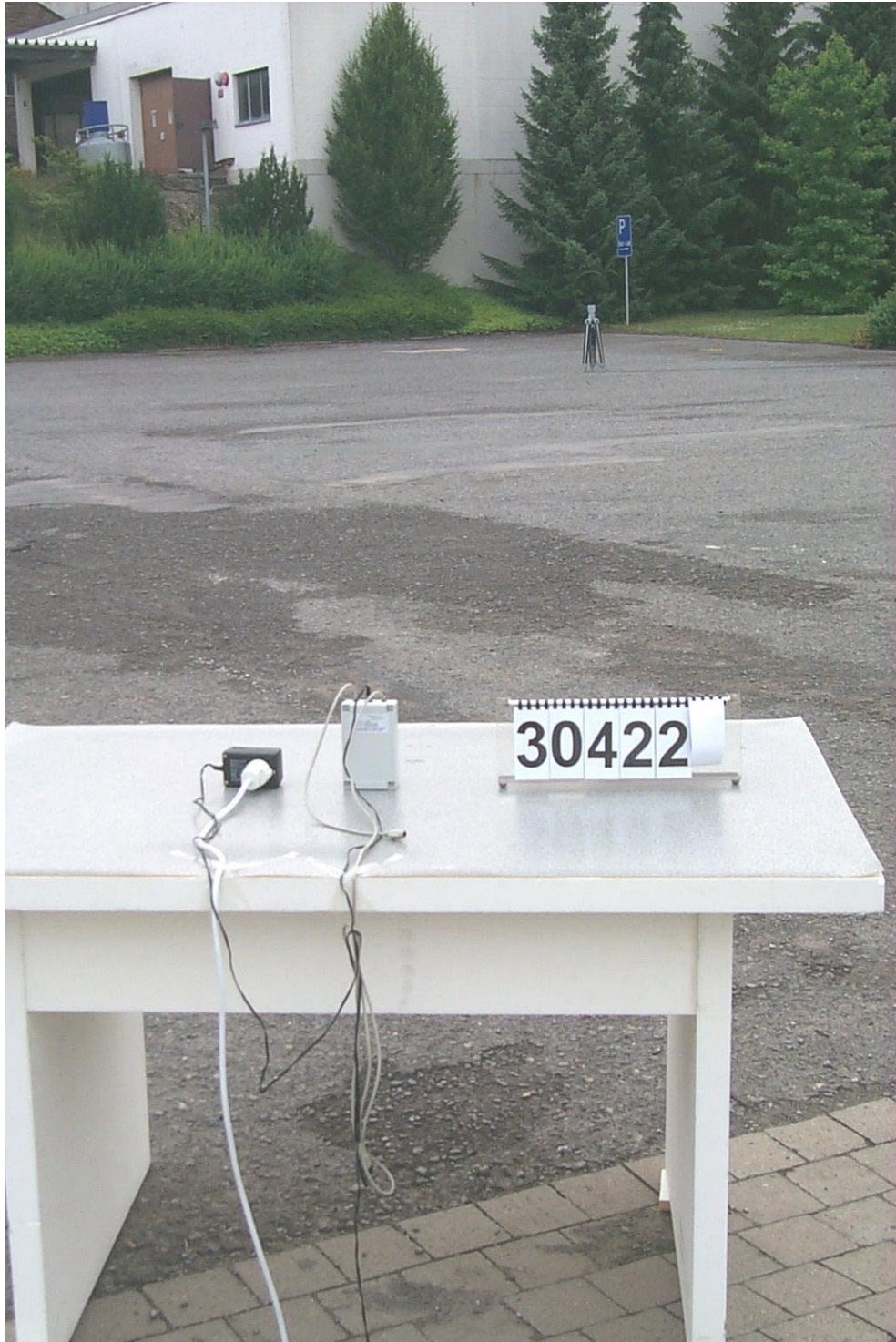
30422_c.jpg Model 24W test set-up final emission measurement (9 kHz to 30 MHz)
