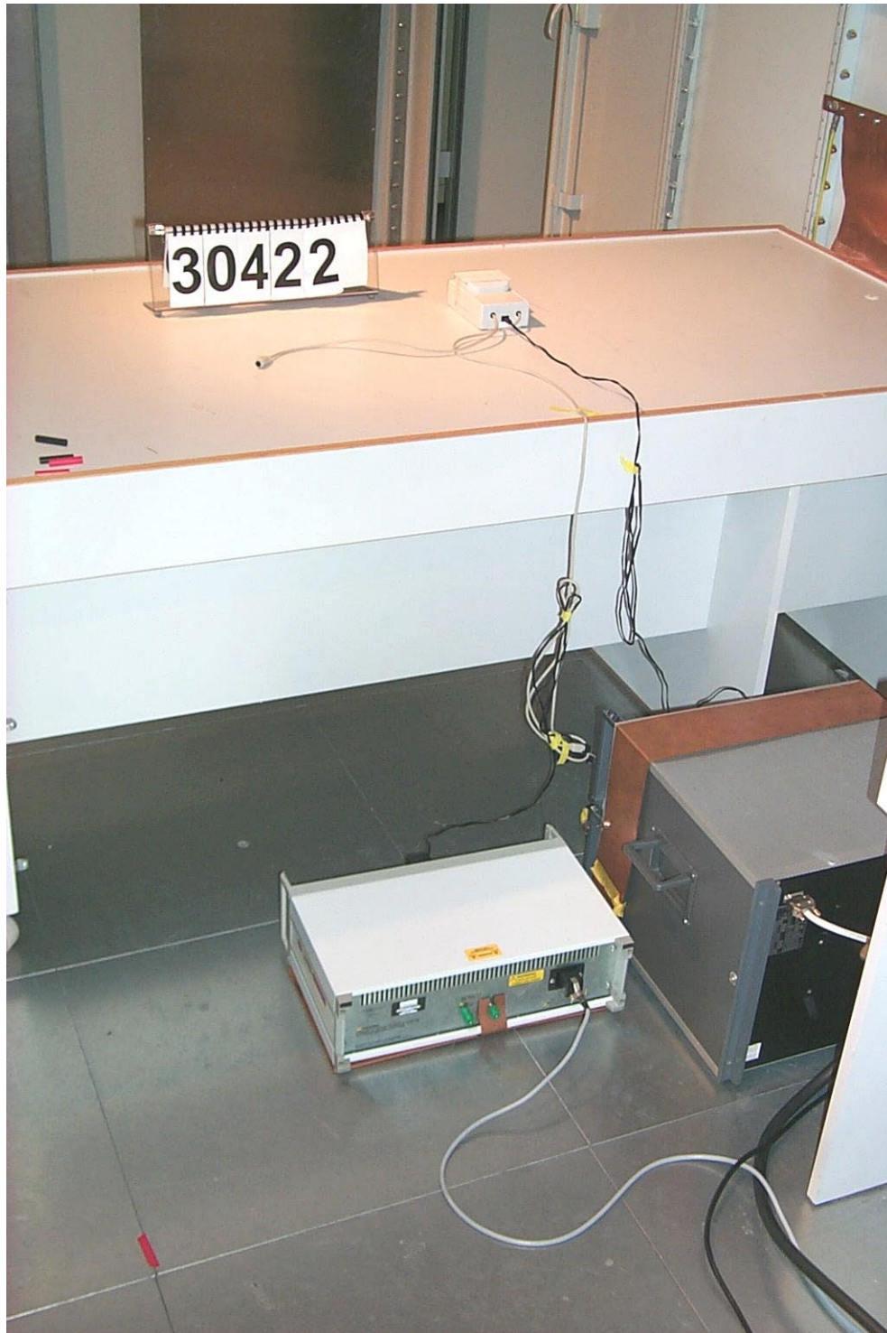
30422_j.jpg Model 24W test set-up conducted emission measurement (150 kHz to 30 MHz)
