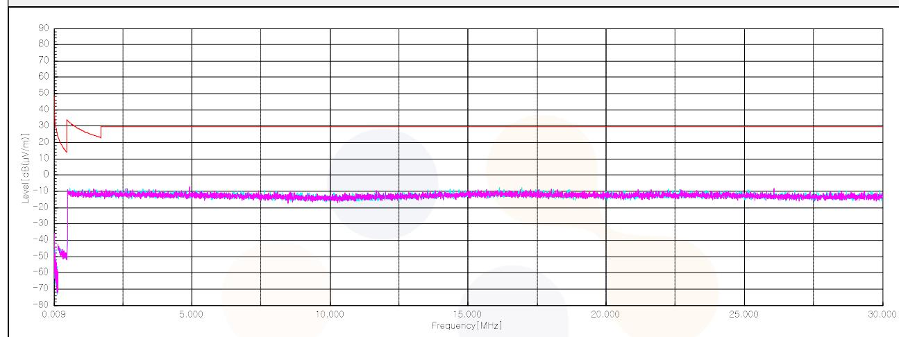
**Test results (Below 1 000 MHz) – Worst case: 802.11n HT20 / 2 462 MHz**
