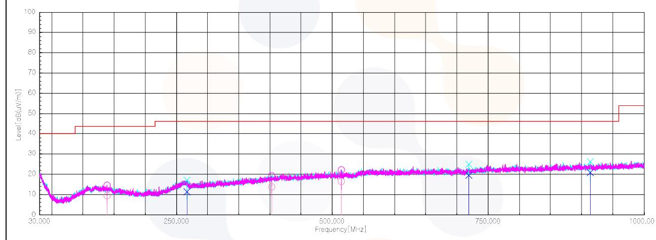
**Test results (Above 1 000 MHz)****802.11b\_2 412 MHz**
