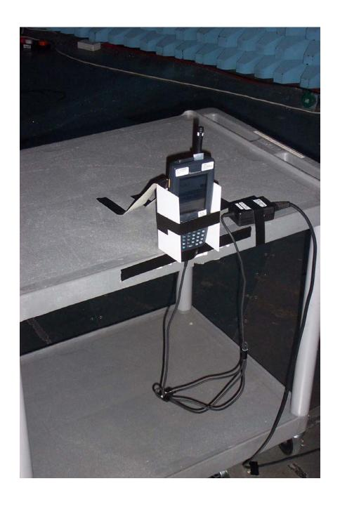
700C - Radiated Emissions Test Setup
