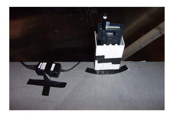
700C - Conducted Emissions Test Setup
