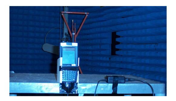
700C - Radiated Emissions Test Set-up
