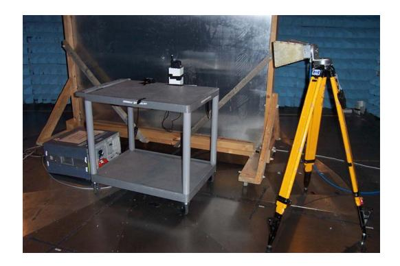
700C - Conducted Emissions Test Setup
