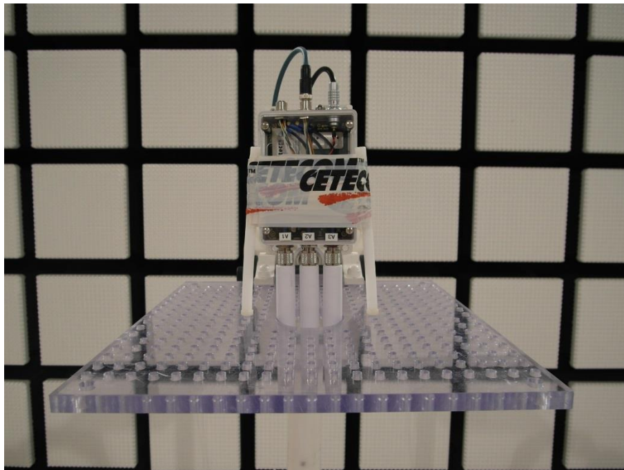
Photo 3 - Measurement Chamber A – Tekfun Dipole Antenna:
