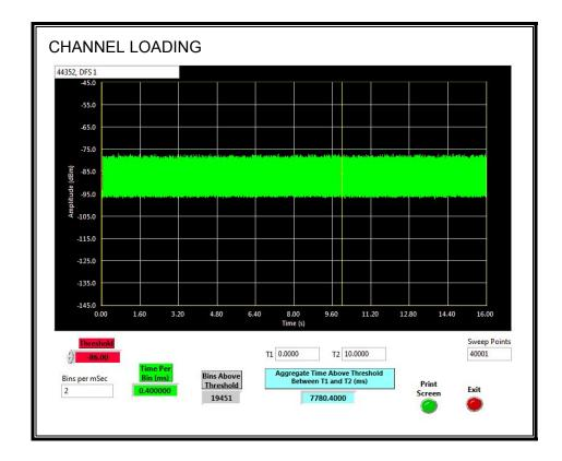
The level of traffic loading on the channel by the EUT is 77.804%.
