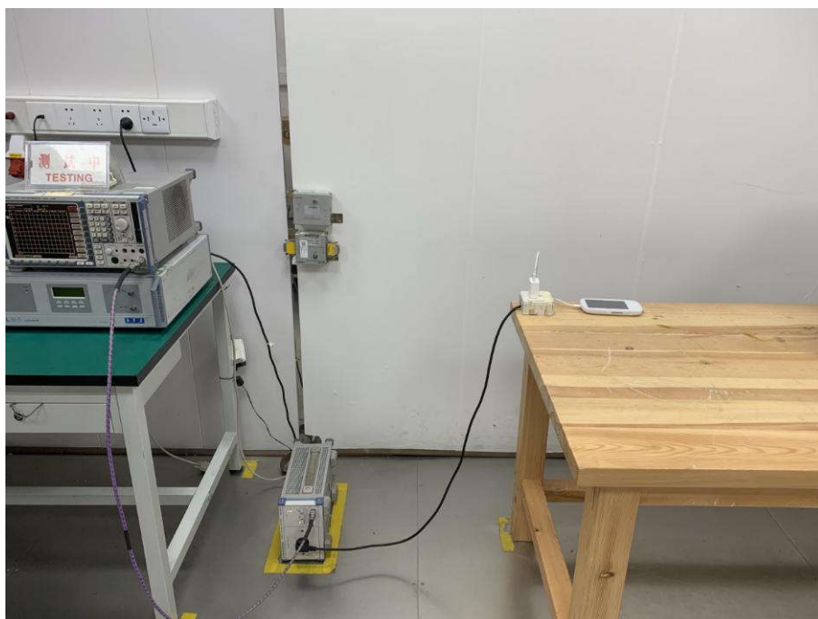
Conducted Emissions Test Setup-4
