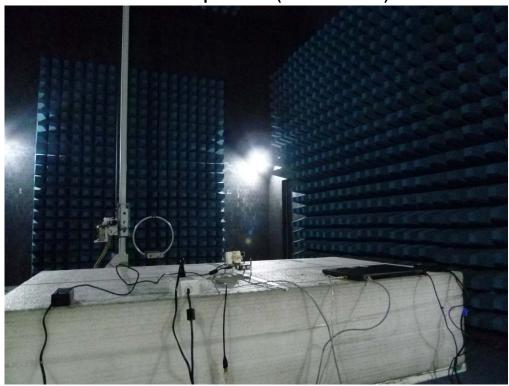
Radiated Emission Set up Photos (Below 1GHz)
