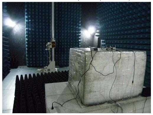
Radiated Emission Set up Photos (Front View)
