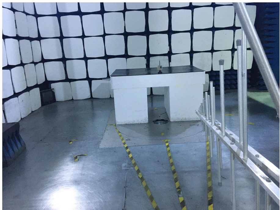
Radiation Emission Test Setup (30MHz to 1GHz)
