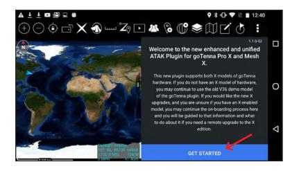
When you first open the goTenna Plugin in ATAK, you'll be prompt to onboard your goTenna Pro-X device and follow a quick tour of the available ATAK features.
