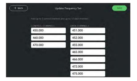
On this page you can change Control and Data channels. By tapping SAVE Frequency Set can be saved.
