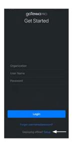
Launch the goTenna Pro app and tap Setup next to deploy offline at the bottom of the login screen.
