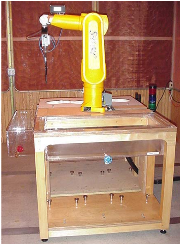
DASY4 SAR Measurement System with validation phantom
