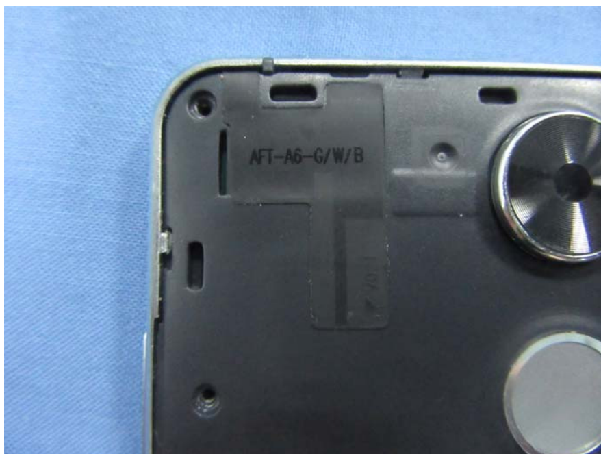
EUT – BT&Wifi Antena View
