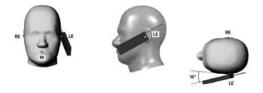
Figure 2 – Phone position 2, "tilted" position. The reference points for the right ear (RE), left ear (LE) and mouth (M), which define the reference plane for phone positioning, are indicated.
