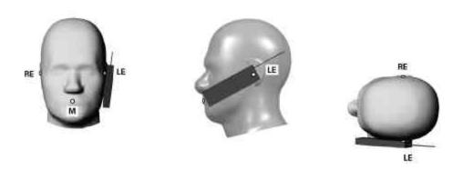
Figure 1 – Phone position 1, "cheek" or "touch" position. The reference points for the right ear (RE), left ear (LE) and mouth (M), which define the reference plane for phone positioning, are indicated.
