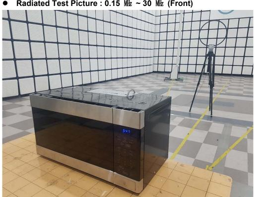
Radiated Test Picture : 0.15 ₩ ~ 30 ₩ (Front)
