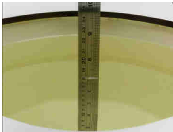
Fig 10.2 Photo of Liquid Height for Body SAR
