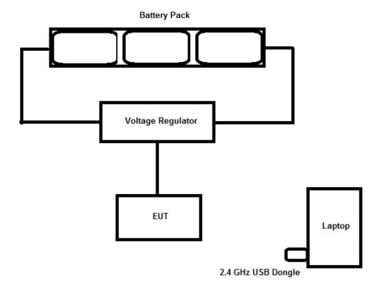
Notes: During testing the battery pack/voltage regulator were located below the ground plane and the laptop was removed from the test setup.
