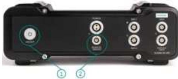
The REMOTE ON/OFF connector (2) allows the UPS Unit to be activated and deactivated by offering an external voltage or by opening or closing a remote switch.
