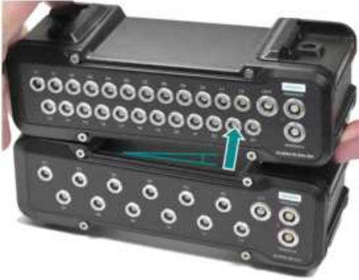
A photograph of two black industrial units stacked vertically. The top unit is being lifted upwards and slightly to the right. A teal arrow points upwards from the top surface of the lower unit towards the bottom of the upper unit, indicating the direction of movement. |
