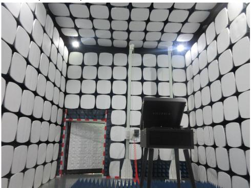
Remark: The transmitter part of the EUT was kept on the high 1.5m above 1GHz according to the lifting platform during the test.
