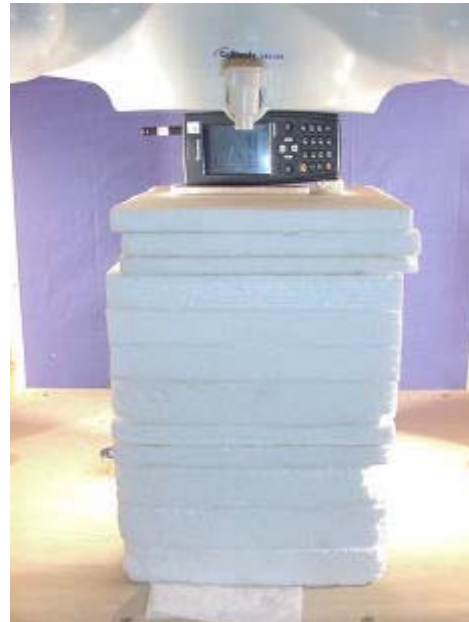
SAR Test Setup Right Side of EUT
