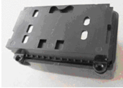
Image 4: Battery Housing Assembly Ready for Screws
