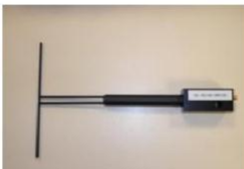
Figure 1 – Satimo COMOSAR Validation Dipole
