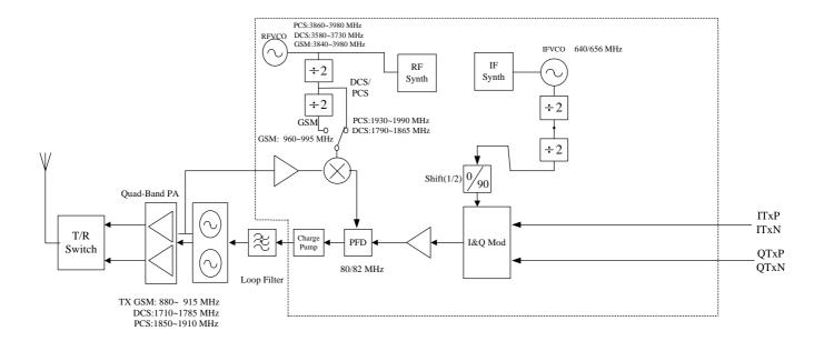
The transmitter chain converts differential IQ baseband signals to a suitable format for transmission by a power amplifier.
