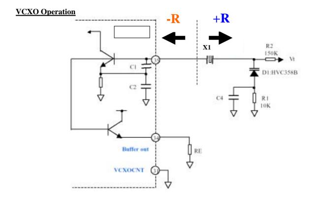
HD155155NP provides a VCXO function. With that function, we can build a reference clock generation circuits as shown in the above graph. This means that the VCTCXO module is not necessary for clock application, and only one crystal with 8ppm tolerance and one varactor are enough.
