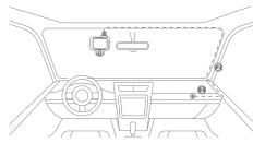
Step 1: Connect the power cable of the device with the B+. ACC and GND power from th vehicle fuse box. For locations, please refer to Figure ①. Step 2: Install the power cable onto the top center of the front windshield along the A-pillar
