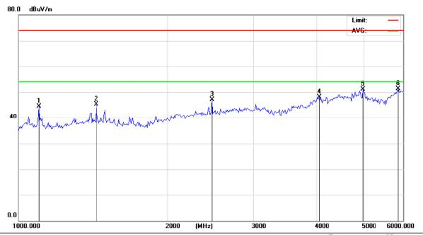
Site Polarization: Horizontal Temperature: 25 Limit: FCC Part 15B Class B Above 1GHz RE(PK) Power: Humidity: 54 %
