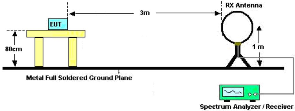
For radiated emissions from 30MHz to 1GHz
