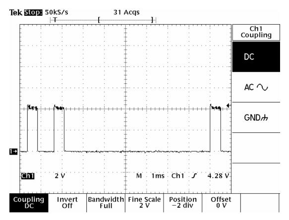
INDIVIDUAL DATA PULSES, QUATERNARY ENCODED DATA FORMAT 500 MICRO SECONDS FOR EACH DATA PULSE TIME DURATION FOR EACH PULSE IS FIXED
