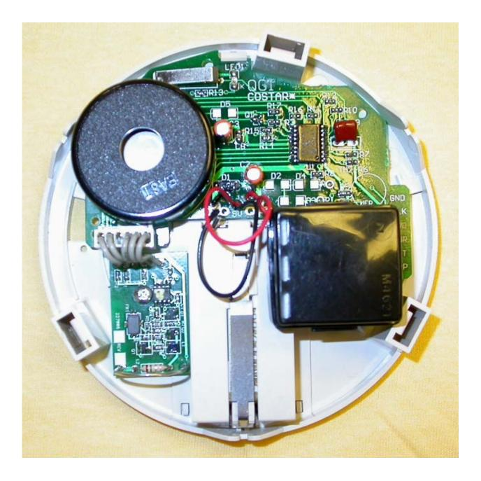
INTERNAL PCB LAYOUT WITH RF TRANSMITTER PCB
