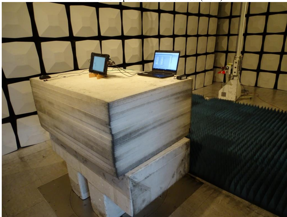
Back View of Spurious Emission Test (Horn)
