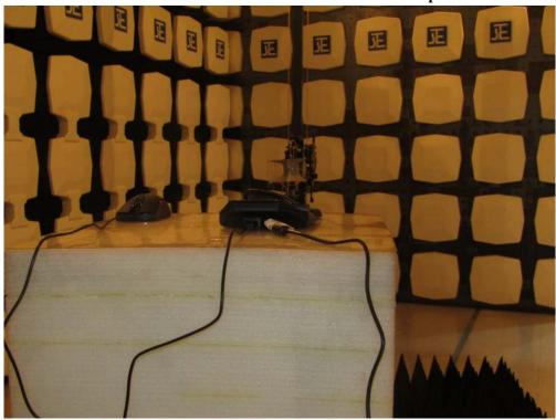
**Measurement of Conducted Emission Test Set Up**
