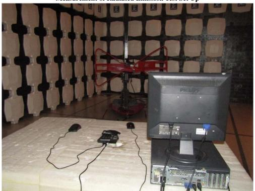
Measurement of Radiated Emission Test Set Up
