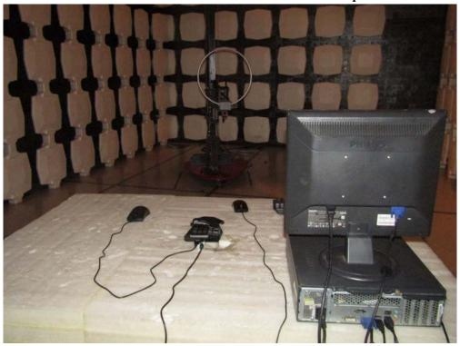
Measurement of Radiated Emission Test Set Up
