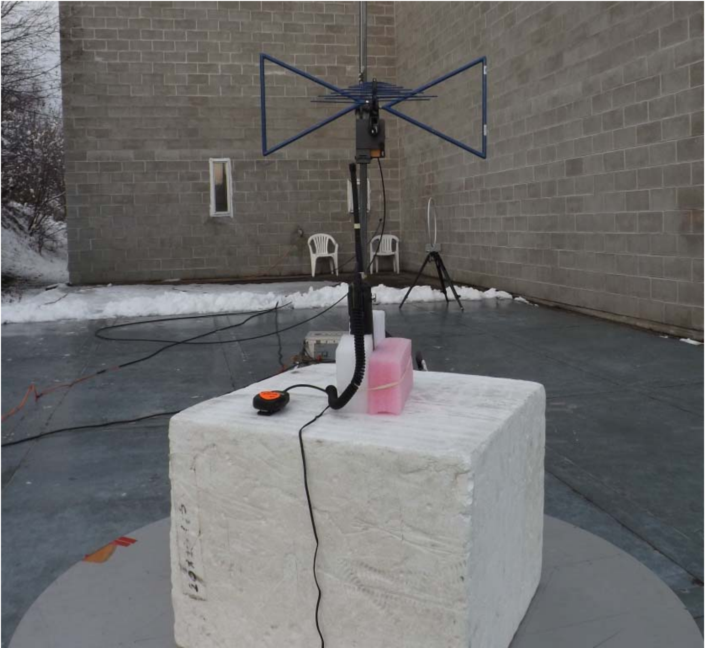
Figure E19.9 – Setup Photo – Radiated Emissions 30 - 1000MHz, Horizontal, With Accessories
