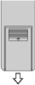
**2** Load two AAA batteries, taking care that the + and - ends face the correct direction.
