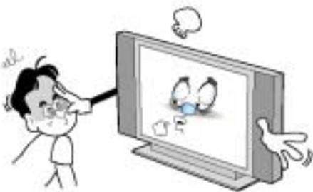
The distance between eyes and the screen should be about 5~7 times as long as diagonal length of the screen.
