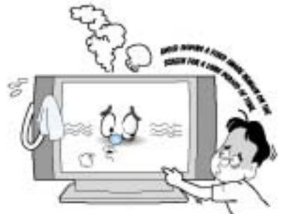
**Avoid having a fixed image remain on the screen for a long period of time. Typically a frozen still picture from a VCR, 4:3 picture format or if a CH label is present; the fixed image may remain visible on the screen.**
