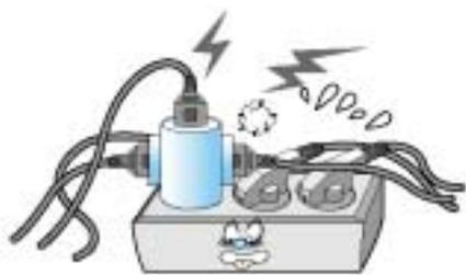
Do not overload the wall outlet or extension cords. Overloading can result in fire or electric shock.
