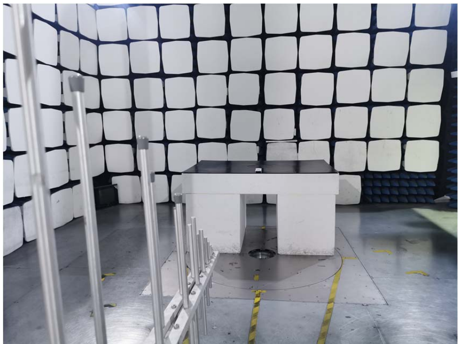
Radiation Emission Test Setup (30MHz to 1GHz)
