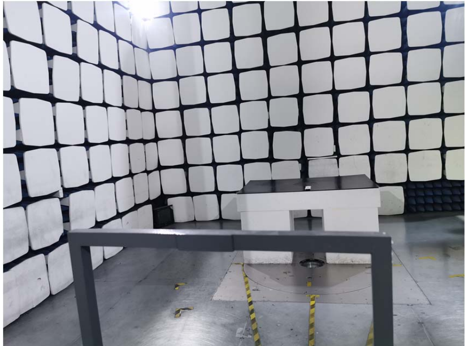
Radiation Emission Test Setup (Below 30MHz)
