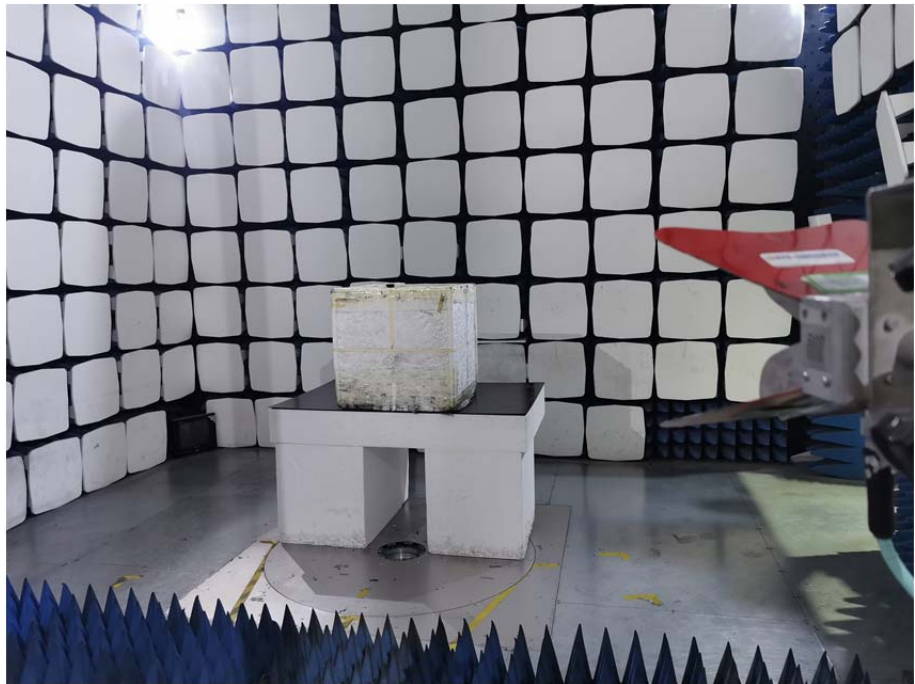
Radiation Emission Test Setup (1GHz to 18GHz)
