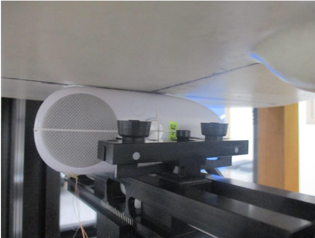
Right Side from Flat Phantom (Separation Distance: 0 cm) – Body SAR
