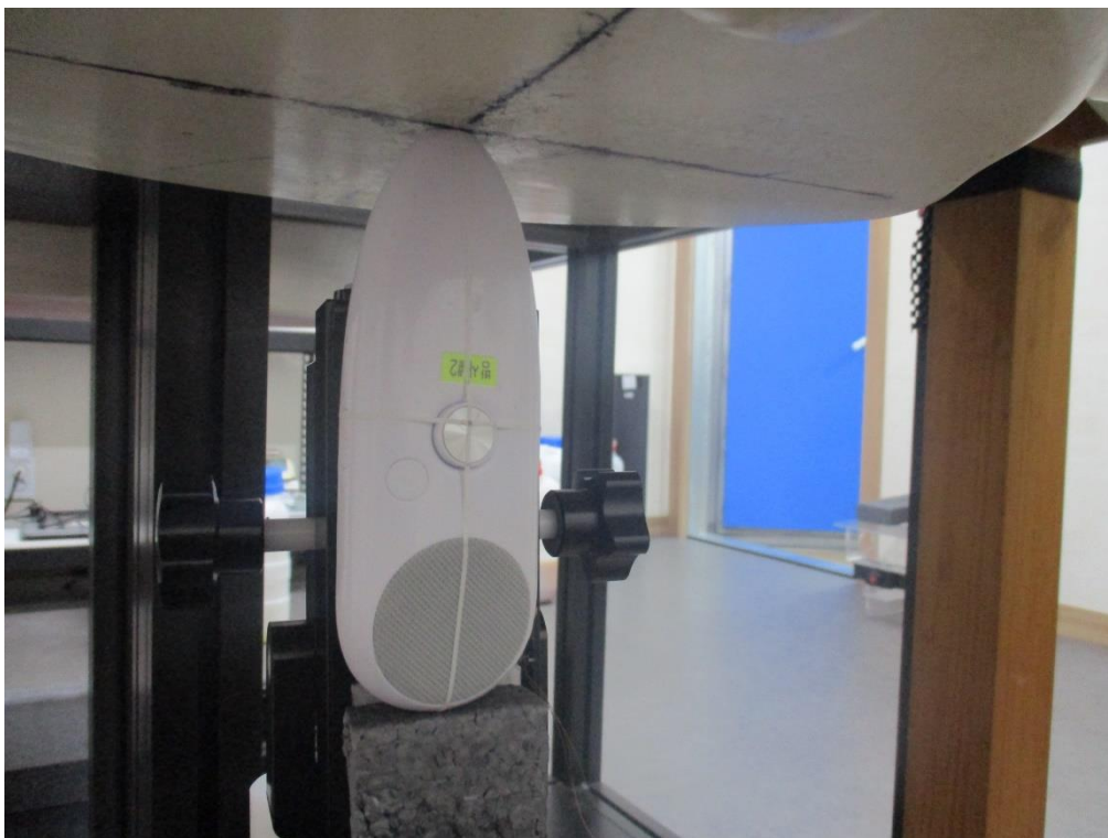
Bottom Side from Flat Phantom (Separation Distance: 0 cm) – Body SAR
