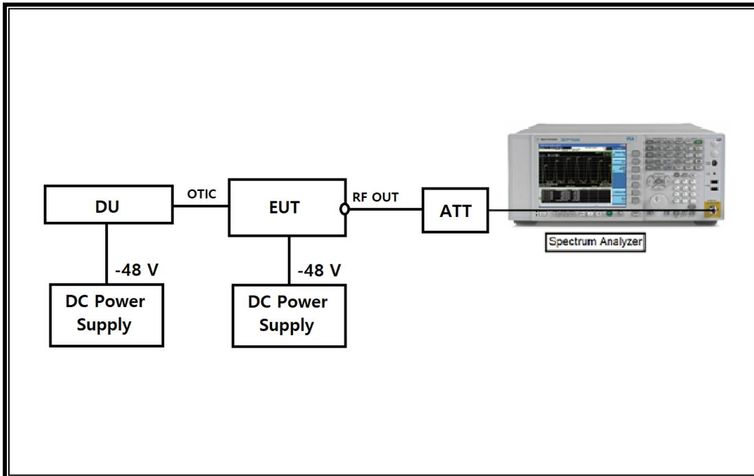
**SETUP DIAGRAM FOR TESTS (RADIATED TEST SETUP)**
